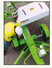
Retractable axles allow the 120 to pass through a 1.10m (3ft 7in) wide opening.
