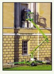
The 120's manual outriggers are both cost effective and simple to set up.
