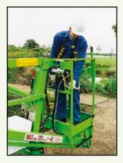
The **Nifty 90** has a telescopic axle allowing it to pass through a 0.75m (2ft 6in) opening and a harness point in the platform for operator safety when working.
