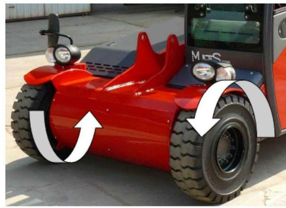
**front wheel drive with 2 motors and counter rotation - total steering**
