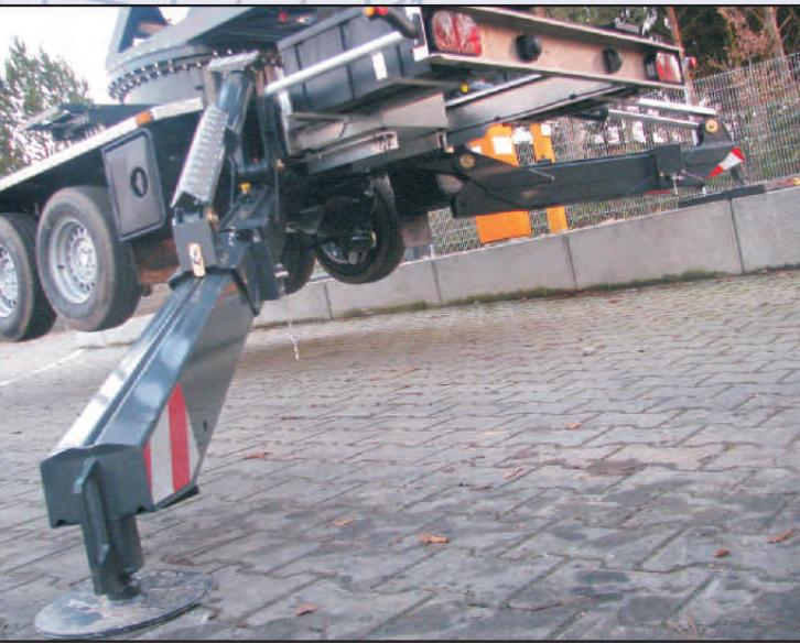
Flexible configuration with single fold-away outriggers
