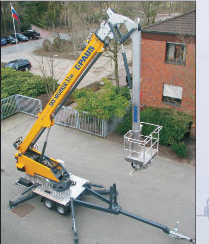
Optional working basket add-on with a working height of 27m
