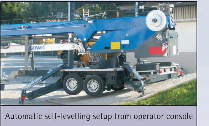
Automatic self-levelling setup from operator console
