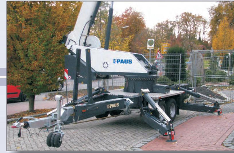
Compact machine with retractable tow-bar
