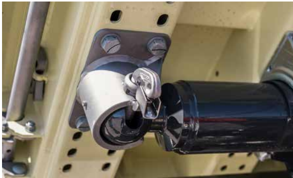
Ball-type tipping parts for one-hand operation
