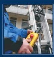
control and end cut-off for smooth start and stop of the furniture platform, as well as spring cable drum with sliding contacts
