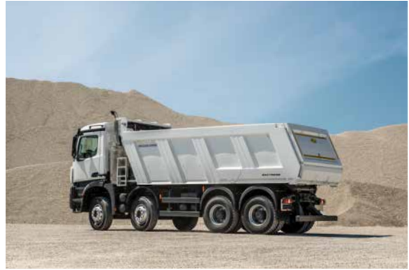
MAXTREME rear tipper with angular tipper body shape.
