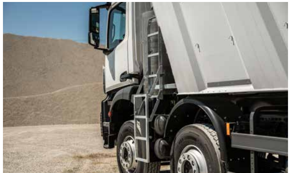
Quickly folded out: climb up the side using the access ladder.
