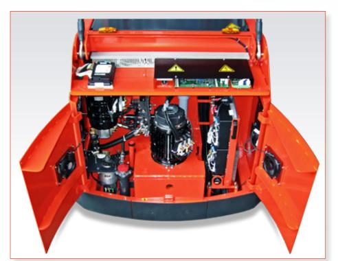
Controls can be accessed without truck specific tools or software. All models have the same board layout. This allows exceptional parts interchange ability for best possible parts and service support. The design of the control systems allows upgrades to be added even after the trucks have been in operation for years.
