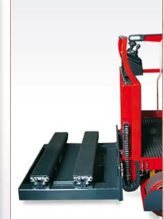
The Telescopic Fork Attachment can operate in smaller aisles, but must use single sided pallets and cannot pick up or deposit from the floor.
