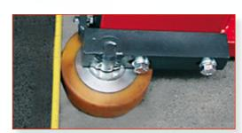
Rail guidance for top speeds in smallest aisles
