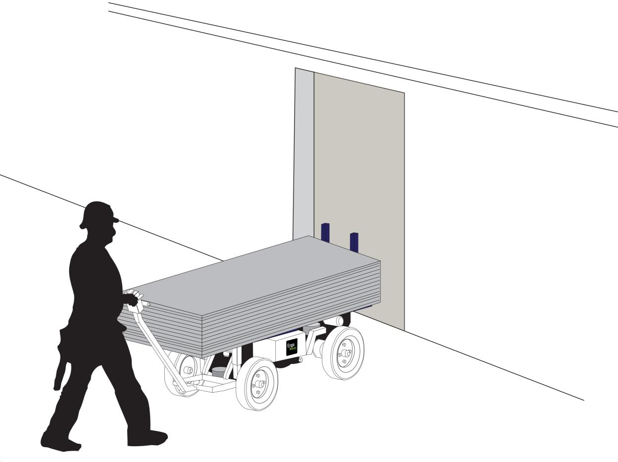
Horizontal unloading of stacks of drywall on trestles or vertical unloading of stacks of drywall in ErgoLoader
