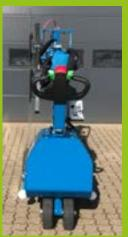
Winlet 400CL is equipped with extra narrow steering and traction wheels and has a width of only 690 mm when the load is on the side of the machine.
