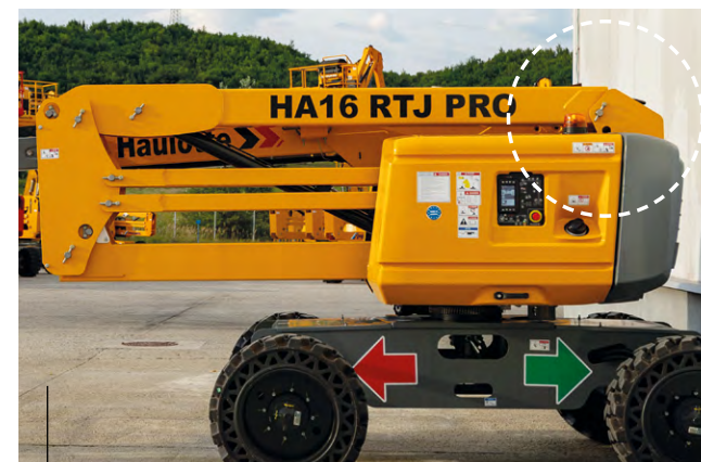
BOOM PROTECTED by the counterweight frame
