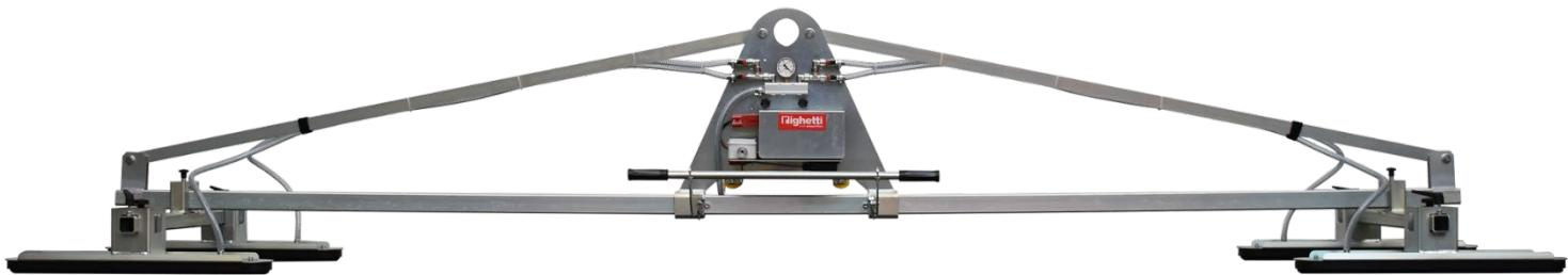
F4B400-CL is a vacuum lifter featuring a horizontally fixed frame, ideal for lifting and handling sandwich panels in workshops and logistic areas. The main fixed crossbeam is available in three different lengths (3000mm, 4000mm, 5000mm) and it's supported by strong high-strength tie rods.
