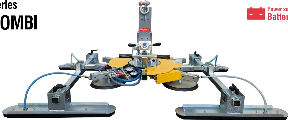
KOMBI is a hybrid vacuum lifter designed for **the installation of glass and sandwich panels** on construction site. The vacuum lifter is powered by high-capacity rechargeable and removable batteries. In compliance with European Laws EN13155, KOMBI is equipped with a dual vacuum circuit and safety devices.
